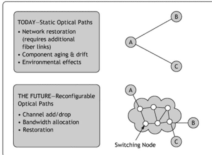
The easily reconfigured “network of the future”—based on dense wavelength division multiplexing (DWDM) technology and characterized by streamlined channel switching, channel add/drop, as well as dynamic path reconfiguration for bandwidth allocation and restoration—requires its components to be similarly flexible. As it pertains to dispersion compensation modules, specifically, *tunability* and inherent *multichannel capabilities* become issues of paramount concern.
