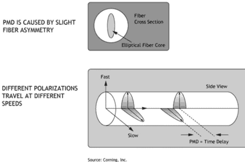
PMD levels rise directly with network speeds (i.e., PMD is four times as severe at 40 Gbps OC-768 as it is at 10 Gbps OC-192) and also increase proportionally to the square root of the distance. For example, if the span length is doubled, PMD increases by a factor of 1.4.
