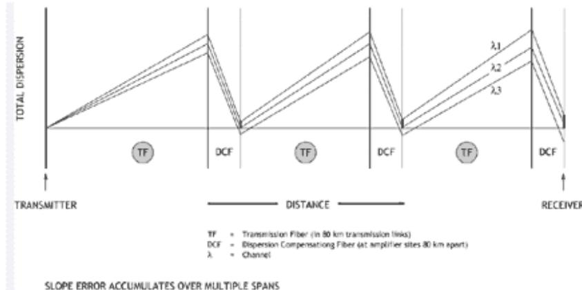
As indicated in *Figure 4*, uncorrected “slope” dispersion at channels away from the center channel ( $\lambda_2$ ) accumulates over successive transmission links and can reach unacceptable levels.
