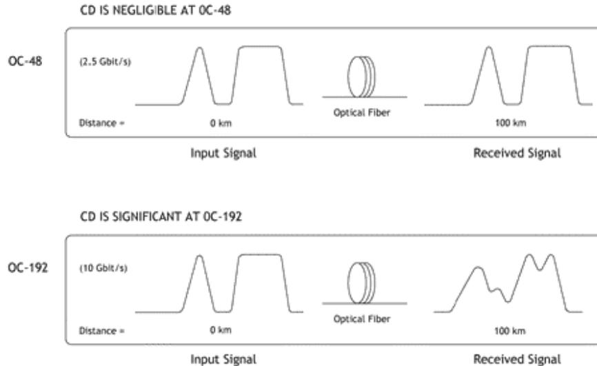
In today's 2.5 Gbps OC-48 networks, the impact of chromatic dispersion is minimal. Unfortunately, dispersion effects do not increase linearly; the growth is at a rate of the square of the increased speed of the transmission. Therefore, at 10 Gbps (OC-192), CD has a major impact on network performance because it is 16 times worse than at 2.5 Gbps (see Figure 3). Similarly, at 40 Gbps, dispersion levels are 256 times higher than at OC-48.
